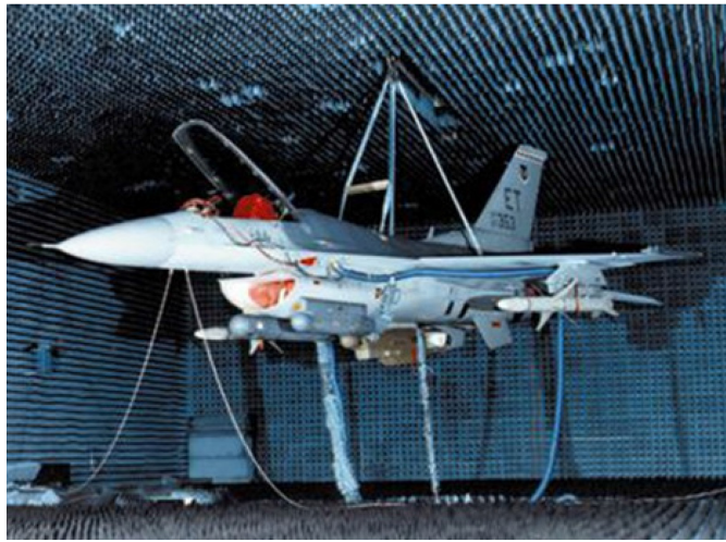
Figure 2-4: F-16 Aircraft preparing for testing in an anechoic chamber [10].
