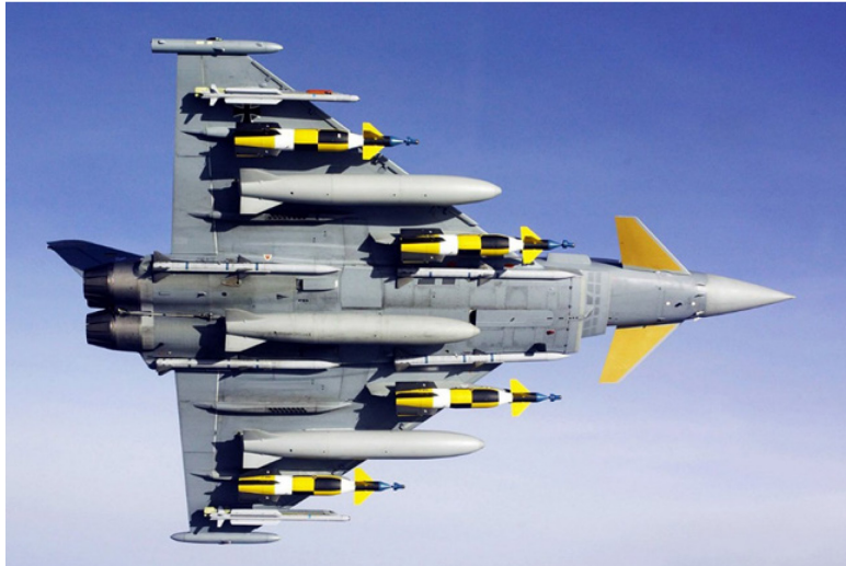
Figure 3-1: Eurofighter loaded with Paveway IV bombs [12].
