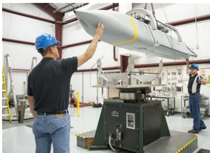
Figure 2-1: Mass properties measurement [6].
